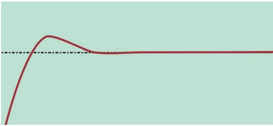
Too Small: Overshoots setpoint before settling
