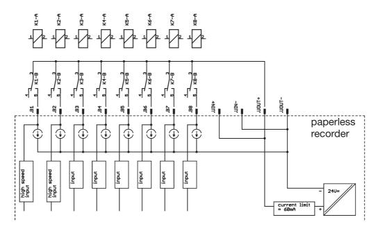
Triggering via external opto-coupler and internal supply voltage:
