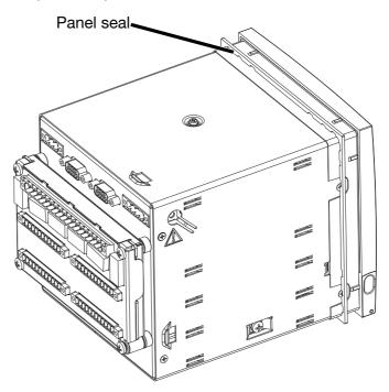
The surface of the panel must be smooth and flat to provide good seating for the panel seal. Check that the seal is evenly and exactly positioned to the front.
