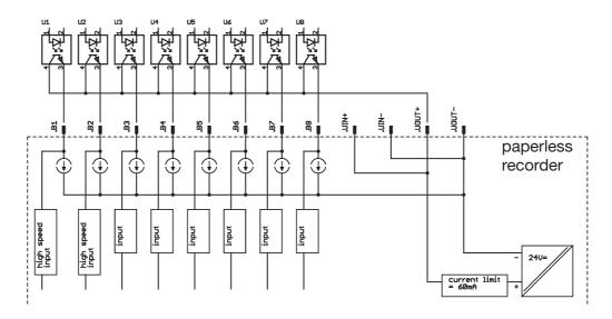
Triggering via external switches (potential-free) and internal supply voltage:
